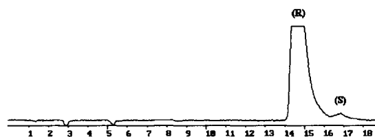
Fig. 8. Determination of enantiomeric purity of ( R )-metoprolol. Solid phase, Hypercarb II; mobile phase, 5 mM L-ZGP and 3 mM NaOH in methanol; column temperature, 0°C; solute, 1% ( S )-metoprolol in ( R )-metoprolol.
